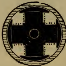
Diagram of magnetic circuit of Siemens & Halske dynamo, 4-pole field inside armature. Leakage coefficient 1.08.
